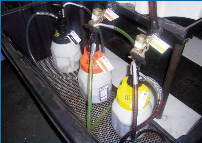
bottles used to transport oil to the units were exposing the oil to contamination. These open and unlabeled containers were also leading to oil mixing, which caused early drain intervals and other problems.
